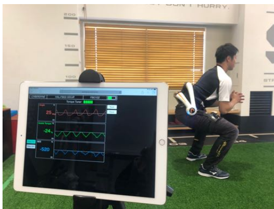
HAL Lumbar Type with Monitor Function (Photo provided by IWA JAPAN)
