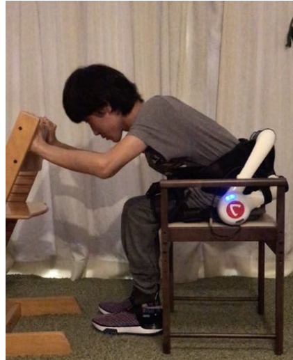
HAL Lumbar Type with Monitor Function (Photo provided by IWA JAPAN)
