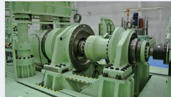
Main shaft bearing test rig for multi-megawatt class wind turbine
