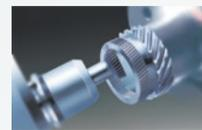
Small-diameter gears created using the skiving process
