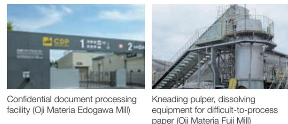
Confidential document processing facility (Oji Materia Edogawa Mill) | Kneading pulper, dissolving equipment for difficult-to-process paper (Oji Materia Fuji Mill)
