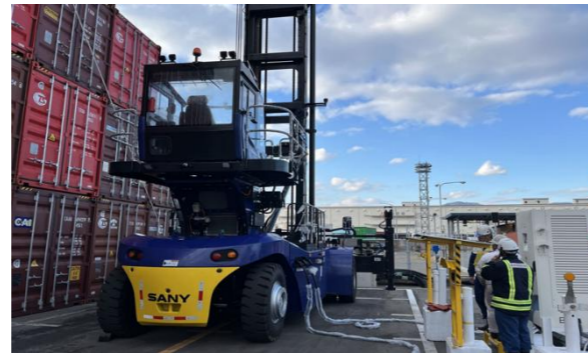
Dual charging possible at charging station (Charge time roughly 1.5 hours, enabling roughly 8 hours of continuous operations)
